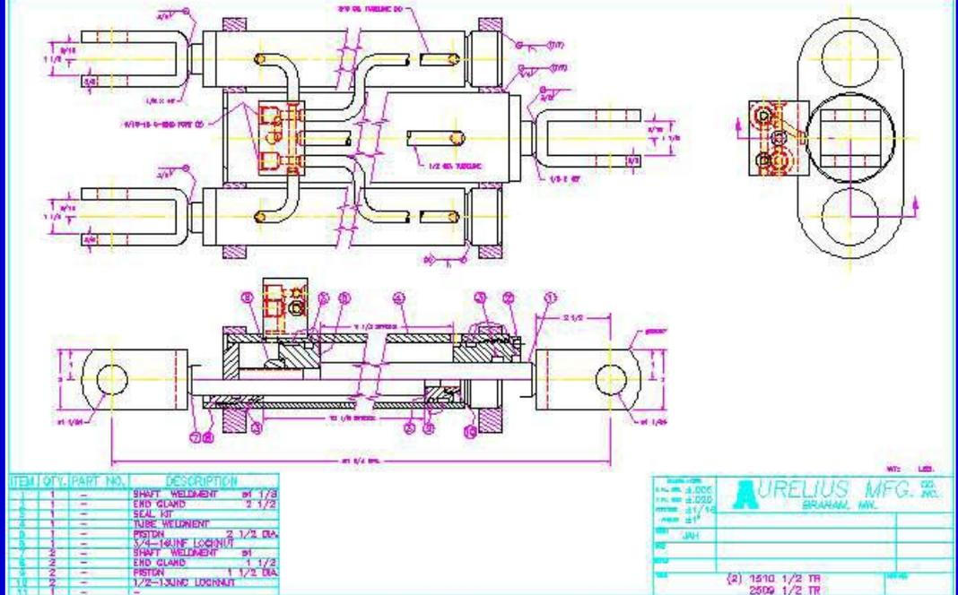
**Requirement:** Provide 20 inches of stroke and a specific mounting configuration that included a closed length of only 21 ¾ inches.
